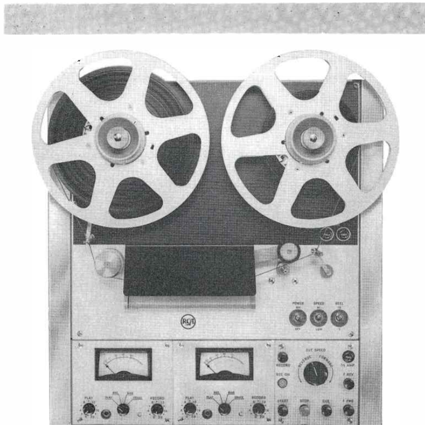
FIG. 1. This is the stereo version of the RT-21A Tape Recorder with two record/play amplifiers mounted side by side. The control unit is on the right. The tape transport unit (above the amplifier panel) is very functional. Straight line tape threading is accomplished without disturbing the hand cover.
