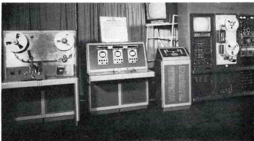
FIG. 3. New TV Tape Editor—developed for NBC by engineers of RCA's Astro-Electronics Division. It facilitates editing of tape programs with a speed and accuracy comparable to present film editing techniques. The television editor may select, view, compare and evaluate groups of frames in tape programs and then select the exact beginning and ending frame of the sequence he wishes to remove or alter.
