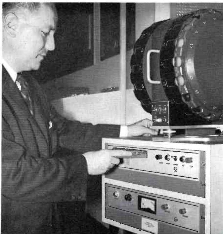
FIG. 10. The "automatic announcer" shown here combines the RT-7 Cartridge Tape Recorder with the TP-7 Slide Projector. The combination will present a complete sequence of slides which are synchronized with and activated by a recorded announcement.
