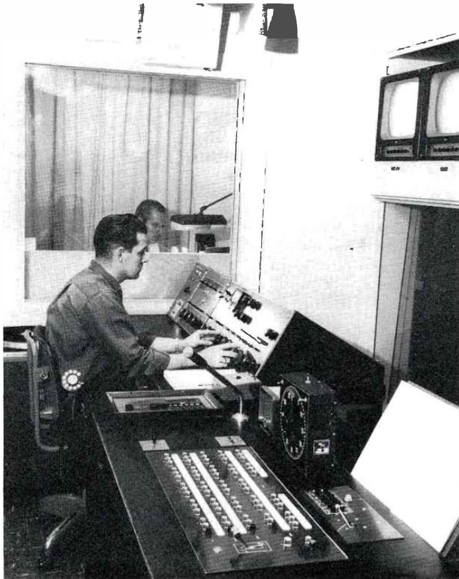
FIG. 17. Sub-control A. In foreground is a panel for TS-40 Switcher. Joe McCrady is operating BC-3 Console. In background is announce booth A.
