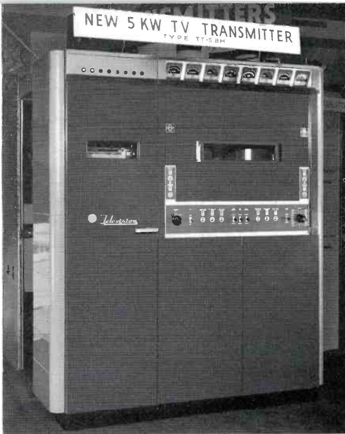
FIG. 11. New 5 kw TV transmitter for high band operation, the TT-5BH is the same size as present RCA 2 kw units. This new compact 5 kw unit is ideal for driving higher power amplifiers and as a standby transmitter. For low power operations, the TT-5BH is an ideal companion for a high gain antenna.
