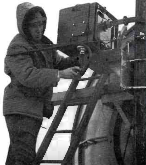
FIG. 2. Carroll Secrist, Chief Engineer, KID-TV, makes last minute adjustments to TVM-1B microwave receiver at the Albion receiving location.
