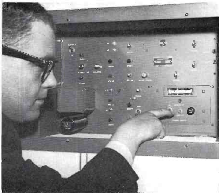
FIG. 5. Sum and difference signal transmission for the new FM stereo system is easily accomplished with the new RCA stereo generator. This compact all-transistor unit generates the supersonic double sideband suppressed carrier AM signal that contains the stereo difference signal. The main channel FM signal is the sum of the two stereo channels, and for receivers not equipped for stereo it sounds like a normal monophonic signal.
